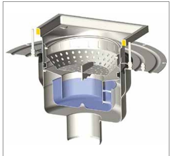
Figure 1. The sealed pocket over the water level in a removable water trap prevents seal failure.
