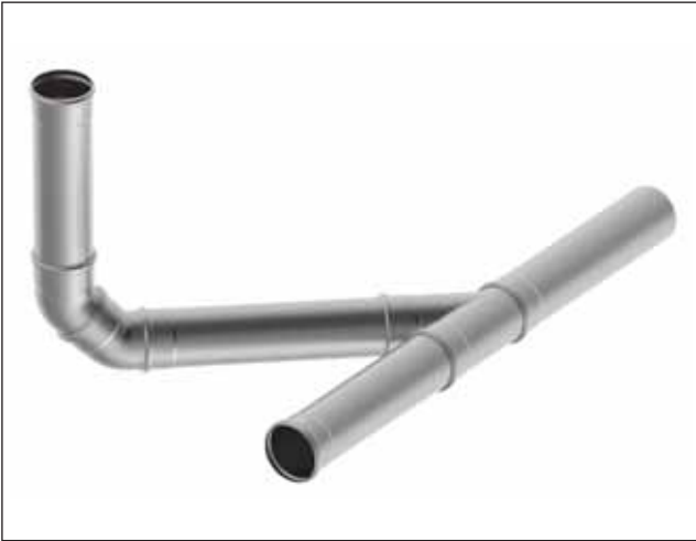
Figure 4. Designing drainage piping with soft 45° bends makes clogging less likely and cleaning easier.
